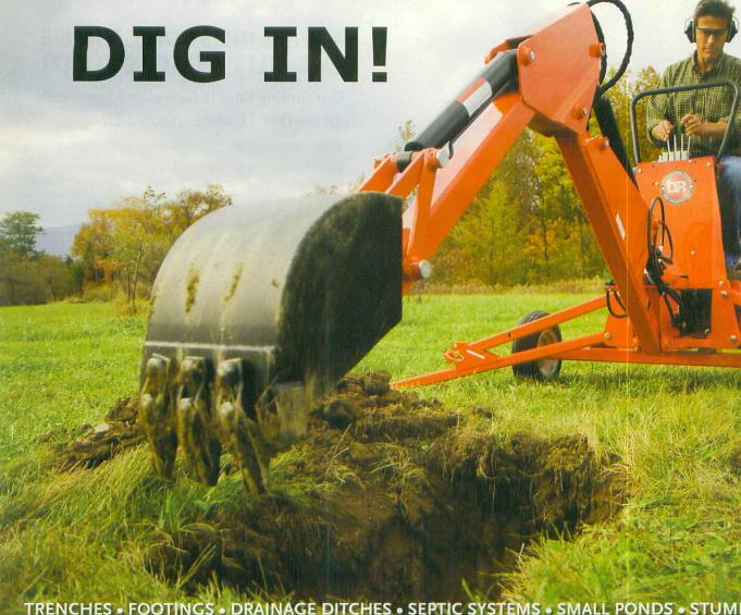
TRENCHES • FOOTINGS • DRAINAGE DITCHES • SEPTIC SYSTEMS • SMALL PONDS • STUMF HOLES FOR TREES • STONE REMOVAL • SPREADING DIRT AND GRAVEL • WATER AND POW
