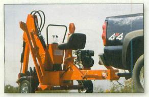
HIGHWAY TOWABLE Using a common 2" ball hitch, the DR\* Towable Backhoe is towable at speeds up to 45 mph.
